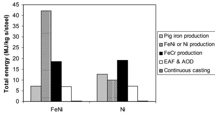
Figure 2. Stage contributions to total energy for stainless steel production.
