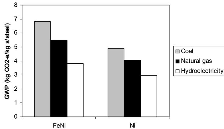
Figure 6. Effect of electricity source on GWP for stainless steel production.
