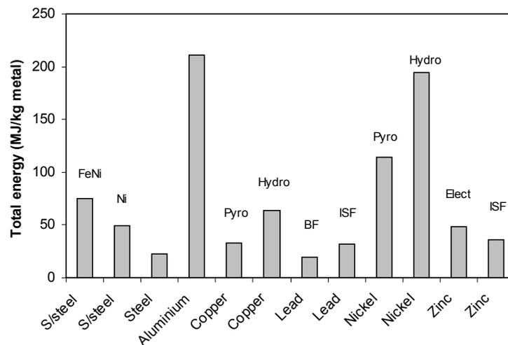
Figure 7. Total energy consumption for stainless steel production compared to other metals.
