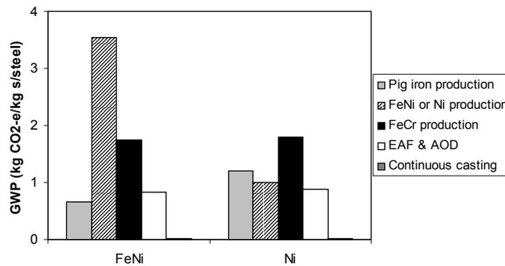
Figure 3. Stage contributions to GWP for stainless steel production.
