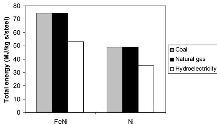
Figure 5. Effect of electricity source on total energy for stainless steel production.
