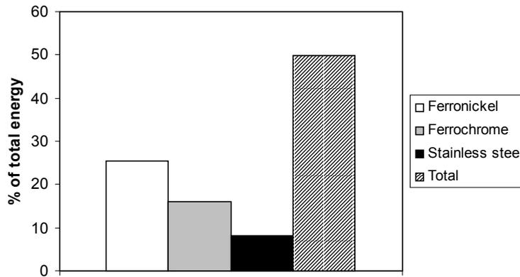
Figure 4. Contribution of electric furnaces to total energy consumption.
