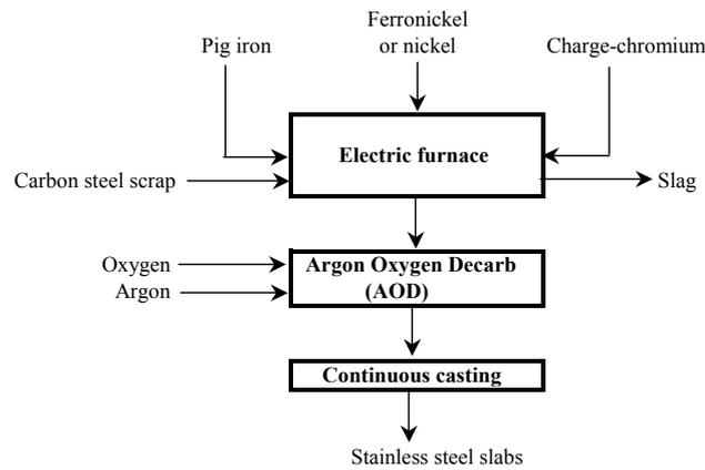
Figure 1. Schematic flowsheet of stainless steel production.
