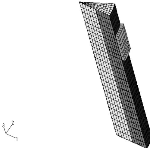
Figure 2. Single Segment of the Electrode.
