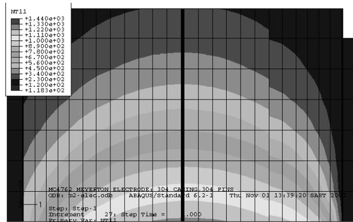
Figure 4. Temperature distribution in contact shoe area of existing electrode [°C]
