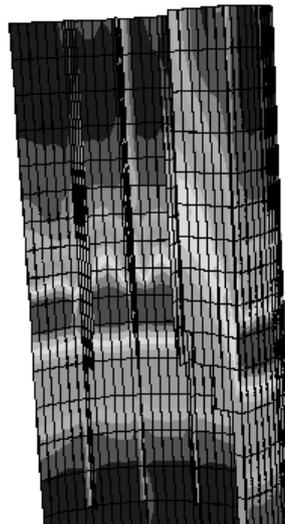
Figure 8. Von Mises Stresses in Steel [Pa].
