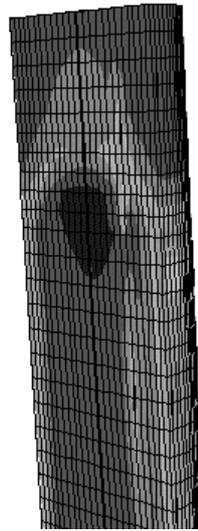
Figure 6. Maximum Principal Stress in Carbon [Pa].
