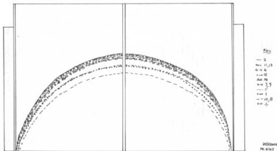
Figure 5. 450°C Isotherm for the Different Material Options.
