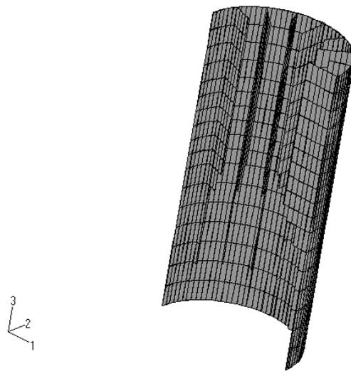
Figure 3. Casing and Fins as Used in Stress Analysis.
