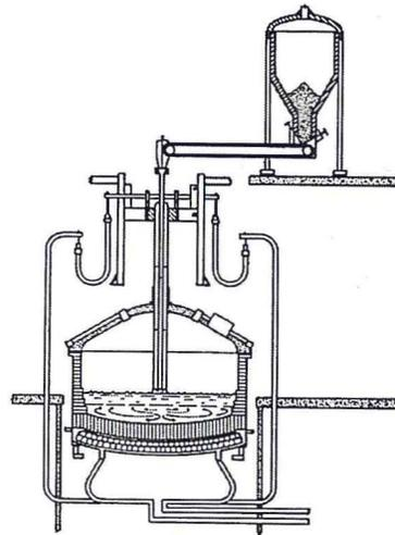
**Figure 2.** Schematic view of the ELRED furnace
