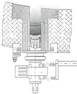
**Figure 7.**The DANIELI water-cooled bottom anode
