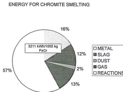
**Figure 9.** Energy consumption for the smelting reactions.
