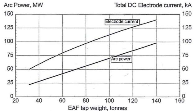
Figure 5. Arc power and total DC electrode current as function of EAF tap weight
