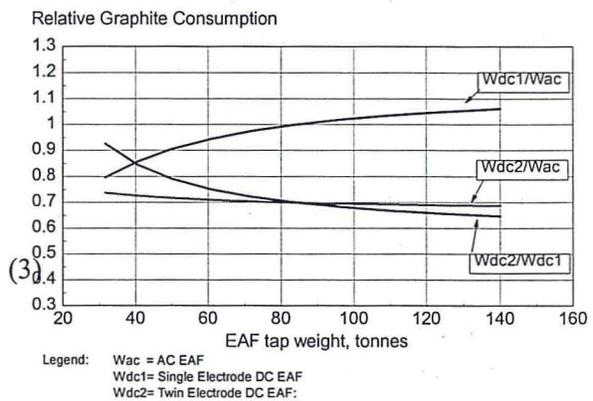
Figure 4. Relative electrode consumption as function of EAF tap weight
