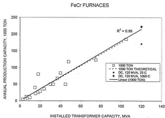
**Figure 10.** Production capacity for FeCr smelters.
