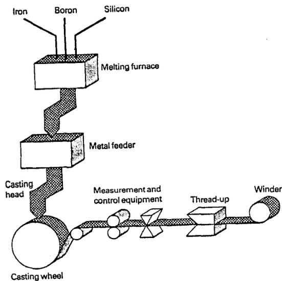
Many thousands of compositions have been studied. The most important, from an industrial point of view, is the 92%Fe 5%Si 3%B (by weight) alloy which has superb magnetic properties making it an ideal material for the core of transformers. There is no doubt it will eventually replace most of the 3% silicon grain-oriented steel now in use.
