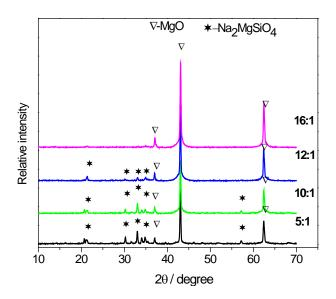
**Fig.3** XRD patterns of the residue from MgSiO<sub>3</sub> after alkali fusion followed by water washing at 600°C for 30 min with different weight ratios of NaOH to MgSiO<sub>3</sub>.
