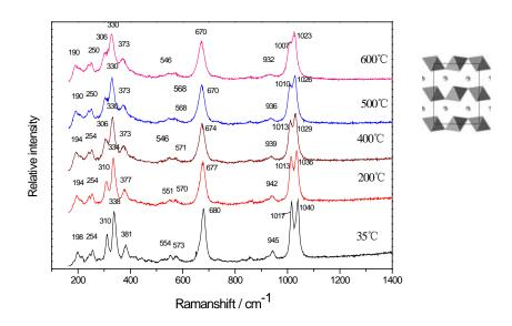
**Fig.2** Raman spectra of prepared MgSiO<sub>3</sub> at varied temperatures from 35 °C to 600 °C.
