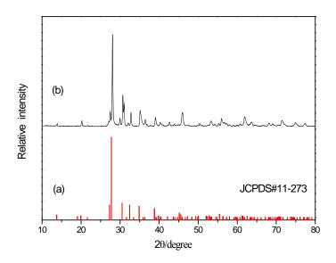
Fig.1 (a) XRD pattern of prepared MgSiO<sub>3</sub> and (b) XRD pattern of protoenstatite (JCPDS No.11-273)
