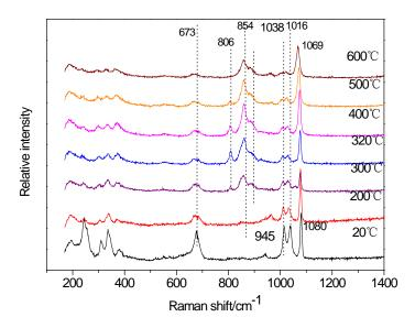
Fig.7 Raman spectra of prepared MgSiO<sub>3</sub> during alkali fusion process as a function of the elevated temperature at mole ratio of NaOH to MgSiO<sub>3</sub> of 2:1.
