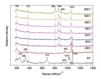
Fig.8 Raman spectra of prepared MgSiO<sub>3</sub> during alkali fusion process as a function of the elevated temperature at mole ratio of NaOH to MgSiO<sub>3</sub> of 5:1
