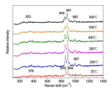
Fig.6 Raman spectra of the prepared MgSiO<sub>4</sub> at different temperatures.
