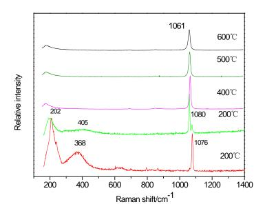
Fig.5 Raman spectra of anhydrous NaOH at different temperatures.
