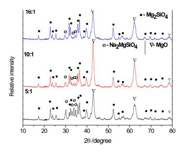
Fig.4 XRD patterns of the residue from MgSiO<sub>3</sub> after alkali fusion followed by water washing at 400°C
