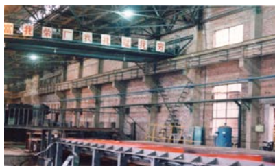
Figure.6 the whole construction of Handan Steel Rolling Mill was completed by steel slag cement
