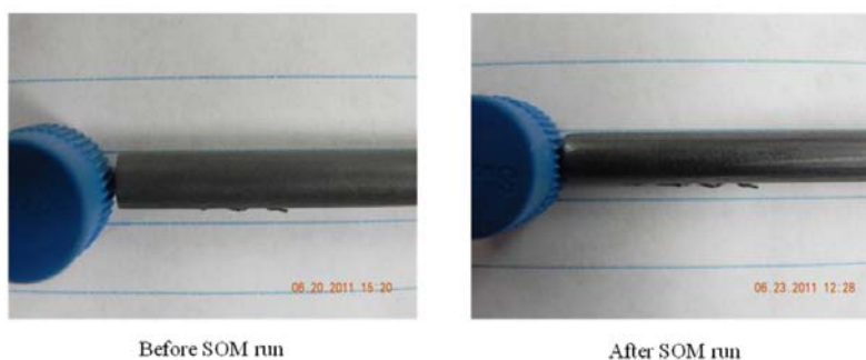
Figure 11. Carbon anode before and after SOM run
