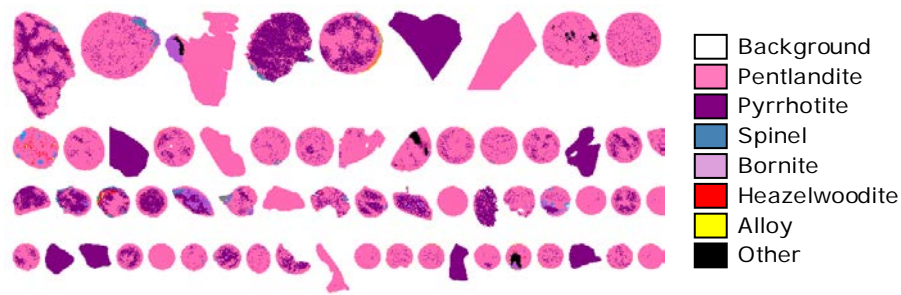
Fig. 6 False colour representation of entrained matte found in slag in section. The largest matte phase shown is approximately 100 \mu\text{m} in diameter
