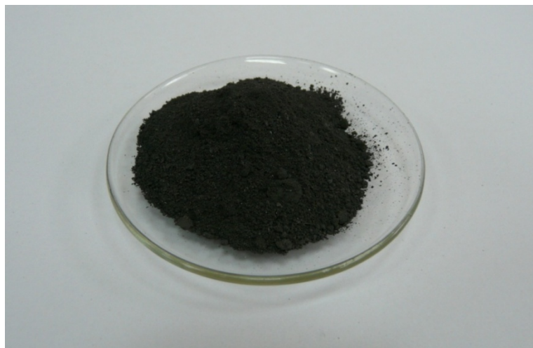
Fig 10. Obtained dusts containing more than 76 wt-% Te.
