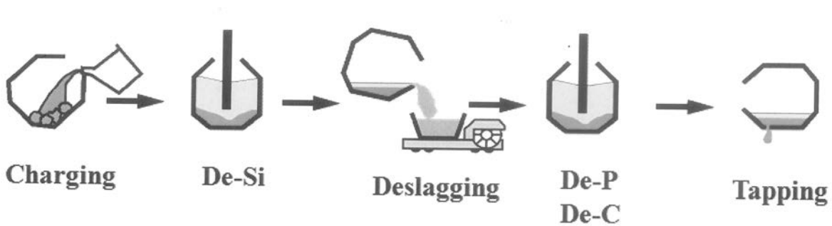
Fig. 1 Outline of double slag process for desiliconization
