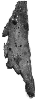
Figure 6: Slag rim, extracted from the mould - Mould powder B, thin slab caster. Right : mould side
