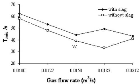
Figure 7: Mixing time variation with gas flow rate at a water bath height of 0.55 m
