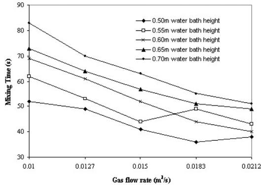
Figure 2: Effect of gas flow rate on the mixing time at different bath heights
