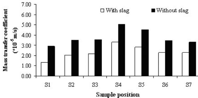
Figure 20: Comparison of mass transfer coefficient values at a gas flow rate of 0.015 m<sup>3</sup>/s near the water bath surface region
