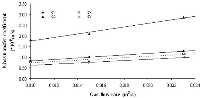
Figure 16: Effect of gas flow rate on mass transfer coefficient at 0.44m bath height
