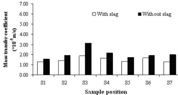
Figure 18: Comparison of mass transfer coefficient values at a gas flow rate of  $0.010 \text{ m}^3/\text{s}$  in the bottom region
