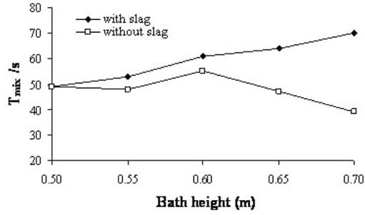
Figure 12: Mixing time variation with bath height at a gas flow rate of  $0.0127 \text{ m}^3/\text{s}$
