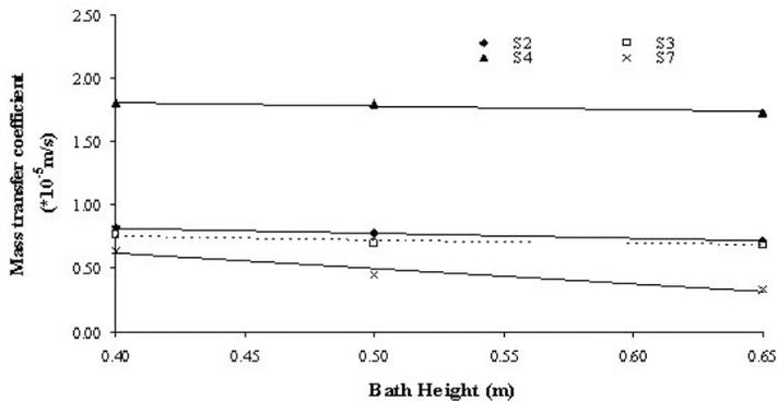
Figure 17: Effect of bath height on mass transfer coefficient at 0.01 m<sup>3</sup>/s gas flow rate
