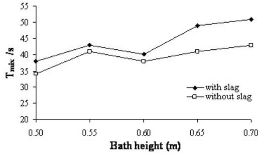
Figure 15: Mixing time variation with bath height at a gas flow rate of  $0.0212 \text{ m}^3/\text{s}$
