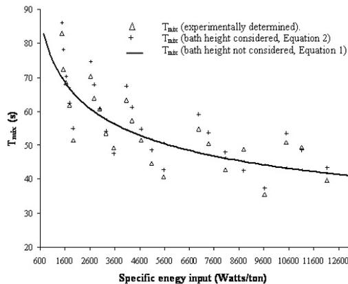
Figure 4: A comparison of the deviations of the estimates from the experimentally determined mixing time values
