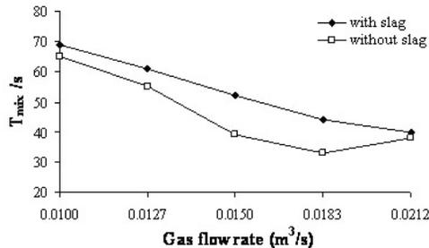
Figure 8: Mixing time variation with gas flow rate at a water bath height of 0.60 m
