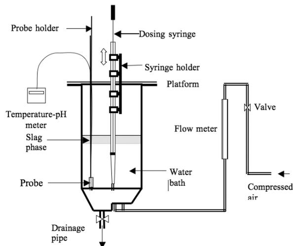
Figure 1: The general set-up of the apparatus used for mixing time measurements Chaendera *et al.* [9]
