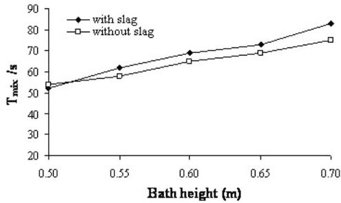
Figure 11: Mixing time variation with bath height at a gas flow rate of 0.010 m<sup>3</sup>/s
