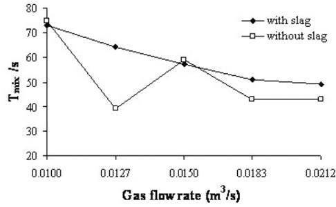
Figure 9: Mixing time variation with gas flow rate at a water bath height of 0.65 m
