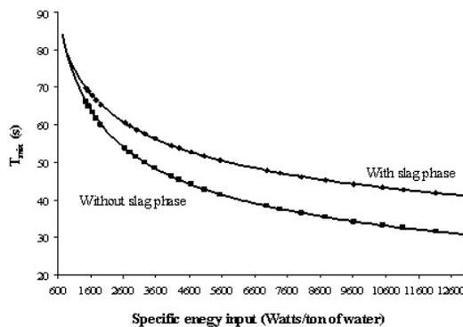
Figure 5: Effect of the slag phase inclusion on the mixing time values predicted for model converter operation
