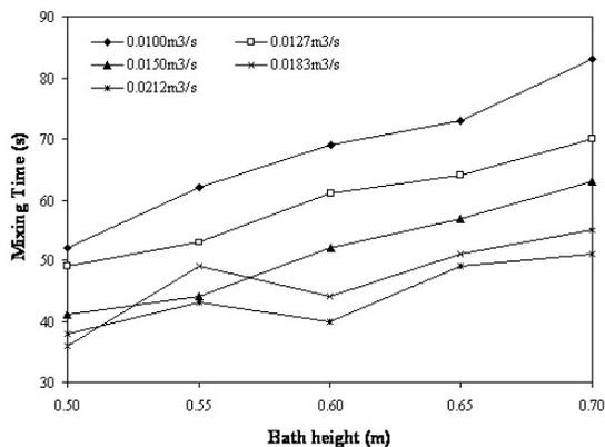
Figure 3: Effect of bath height on the mixing time
