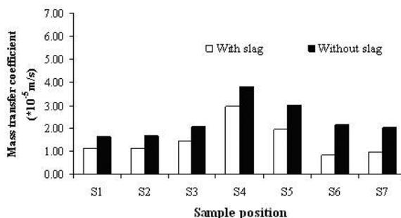
Figure 19: Comparison of mass transfer coefficient values at a gas flow rate of 0.010 m<sup>3</sup>/s near the cone region
