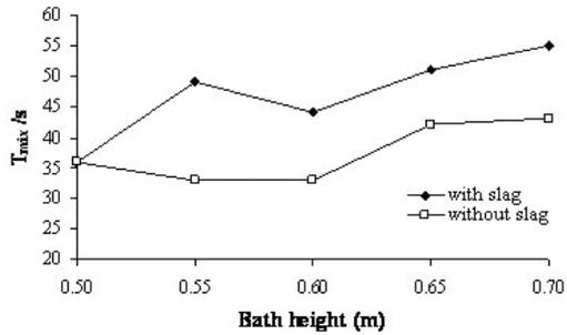
Figure 14: Mixing time variation with bath height at a gas flow rate of  $0.0183 \text{ m}^3/\text{s}$
