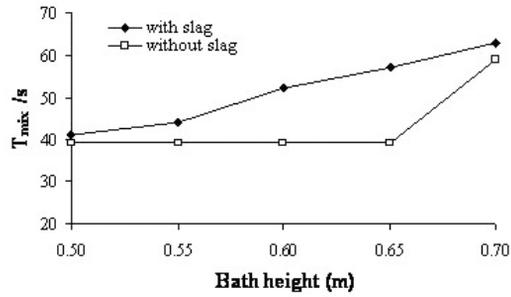
Figure 13: Mixing time variation with bath height at a gas flow rate of  $0.0150 \text{ m}^3/\text{s}$
