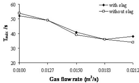
Figure 6: Mixing time variation with gas flow rate at a water bath height of 0.50 m
