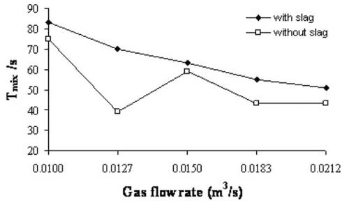
Figure 10: Mixing time variation with gas flow rate at a water bath height of 0.70 m
