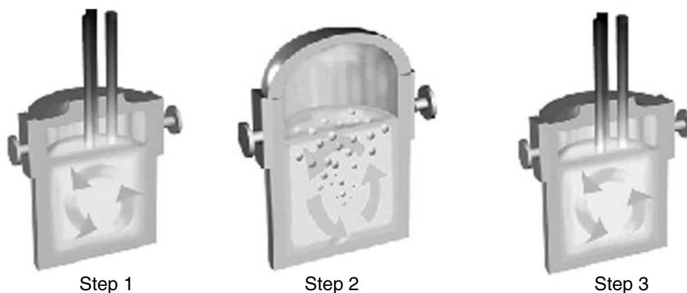
Figure 1. Deoxidation and alloying (step 1), vacuum degassing (step 2), and heating and stirring (step 3)
