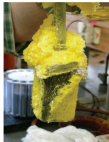
Figure 12—Water-cooled copper specimen coated with sulphur after testing
