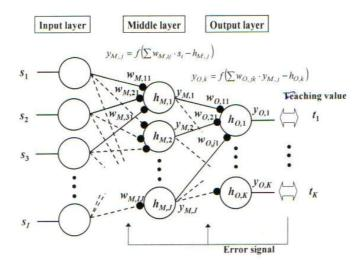
Figure 16: Schematic diagrams illustrating (i) concept of neuron model and (ii) neural network.
