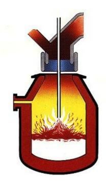
Figure 3: Schematic drawing of BOS process and the turbulence generated which causes refractory erosion
