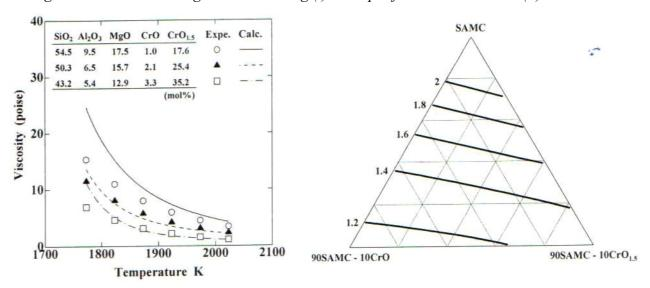
Figure 17: (a) Viscosity as a function of temperature for a MgO+CrO+CrO<sub>1.5</sub>+Al<sub>2</sub>O<sub>3</sub>+SiO<sub>2</sub> slags and (b) Iso-viscosity (dPas) contours for a Fe/Cr process slag at 1923K SAMC=  $(X_{MgO} = 0.41) + (X_{CaO} = 0.074) + (X_{SiO2} = 0.343) + (X_{Al<sub>2</sub>O<sub>3</sub>} = 0.173)$  [22]
