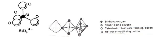
*Figure 9: Structure of SiO*<sub>2</sub> *showing 3-D characteristics*
