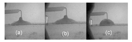
Figure 8: Effect of applying electrical potentials to a molten slag after 2 mins at (a) 0V (b)-1V and (c) -2V
