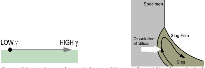
Figure 4: Schematic drawings showing (a) direction of Marangoni flow and (b) mechanism for slag line attack in PbO-SiO2 slag [3]
