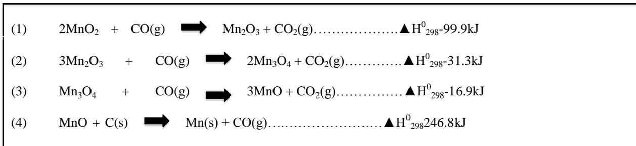
The above reactions (1) – (3) are kinetically controlled for an optimal outcome of producing FeMn/SiMn, and (4) by the thermodynamic environment.
