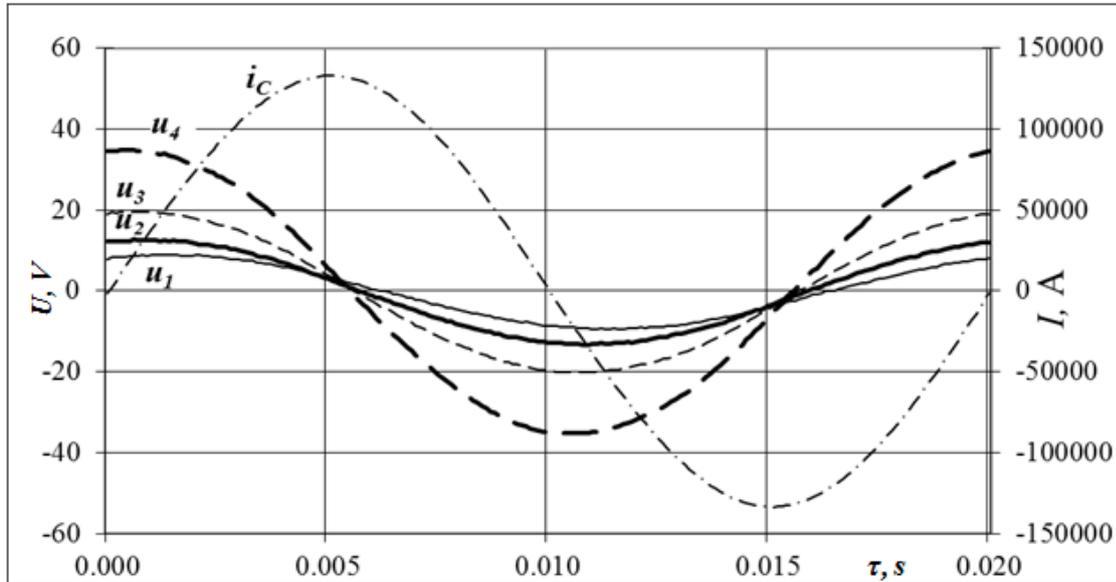
**Figure 2.2:** Curves of operating phase current "C" -  $i_C$  (---) and electrode voltages of non-operating phases induced by it: (—)  $u_1$  is electrode 1; (---)  $u_2$  is electrode 2; (---)  $u_3$  is electrode 3; (---)  $u_4$  is electrode 4, of six-electrode ore-thermal electric furnace.
