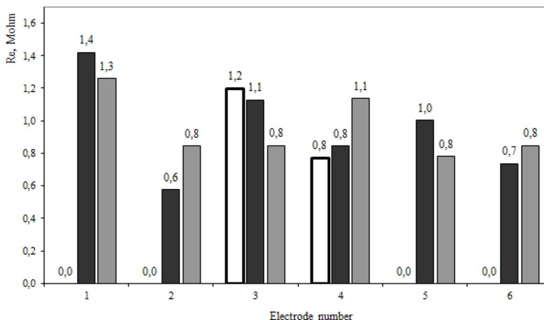
**Figure 4.2:** Values of calculated active resistance of near-electrode space of six-electrode ore-thermal electric furnace: □ - during operation of single phase "B", without effect of neighboring phases current; during three-phase closing: ■ - without correction; ■ - corrected.
