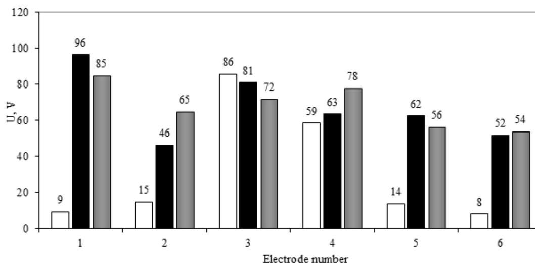
**Figure 4.1:** Values of real electrode voltage values of six-electrode ore-thermal electric furnace: □ - during operation of single phase "B" without effect of neighboring phases current; during three-phase closing: ■ - without correction; ■ - corrected.
