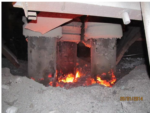
Figure 6: Processing of MnC17 screenings in a continuous process with closed furnace mouth
