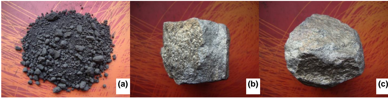
Figure 5: Photograph of (a) the as-received cutting slurry waste, (b) product of Heat 1114-01, (c) product of Heat 1114-02
