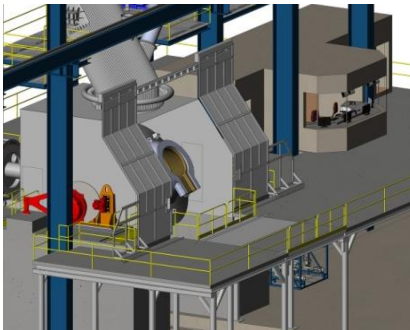
Figure 5: The process control room is here placed to the right of the converter vessel.
