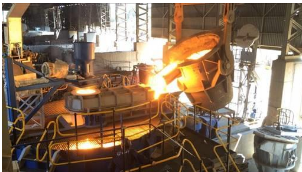
Figure 6: CLU refined FeCr granulated at AFARAK Mogale Alloys plant in SA [8].
