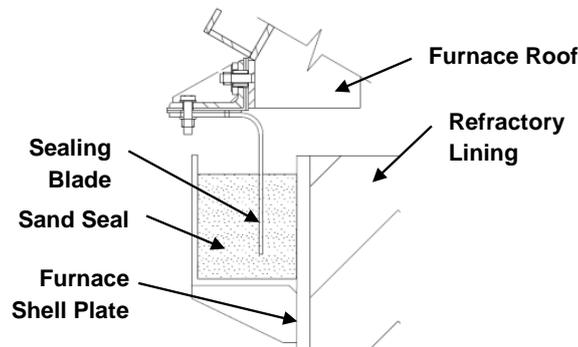
**Figure 6:** Furnace Roof-Wall Sand Seal Simplified Cross-Section
