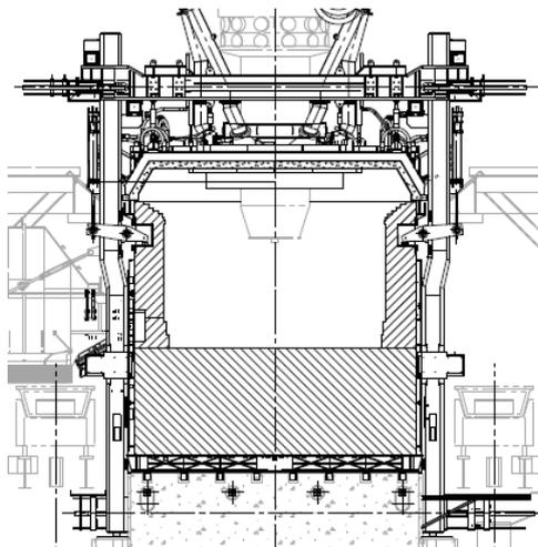
**Figure 3:** Transverse Cross-Section of Furnace
