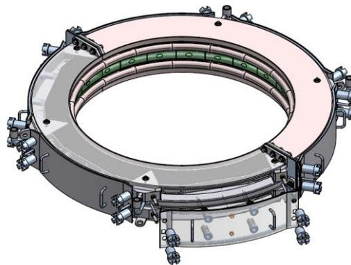
**Figure 7:** Electrode Seal
