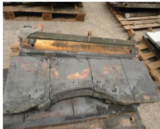
Figure 2: Damaged Coolers Removed from the Furnaces (Original Design by Others)
