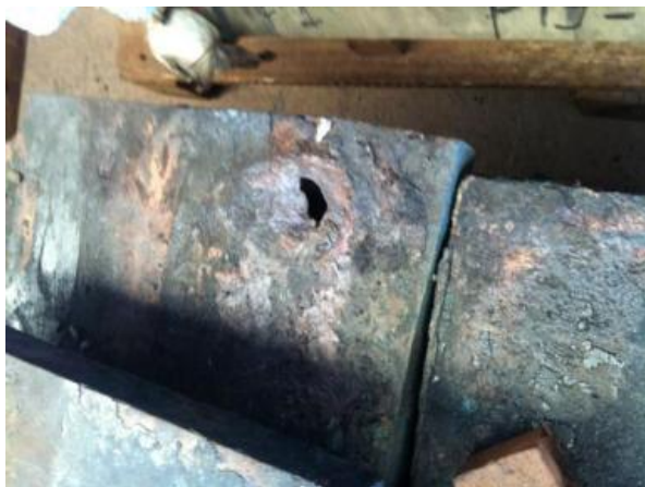
Figure 2: Damaged Coolers Removed from the Furnaces (Original Design by Others)
