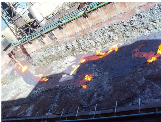
Figure 1: Air cooling of slag in designated areas
