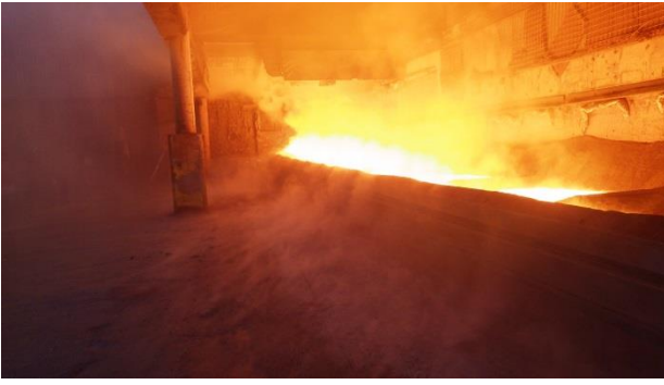
Figure 11: Moisture saturated air being drawn in over the casting beds.
