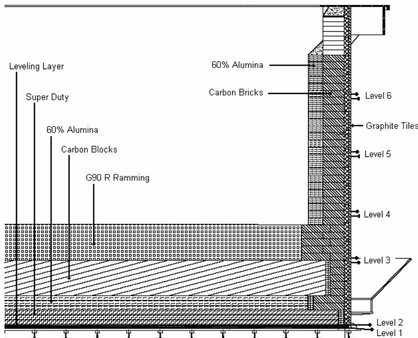
Figure 1: Furnace lining arrangement and materials used
