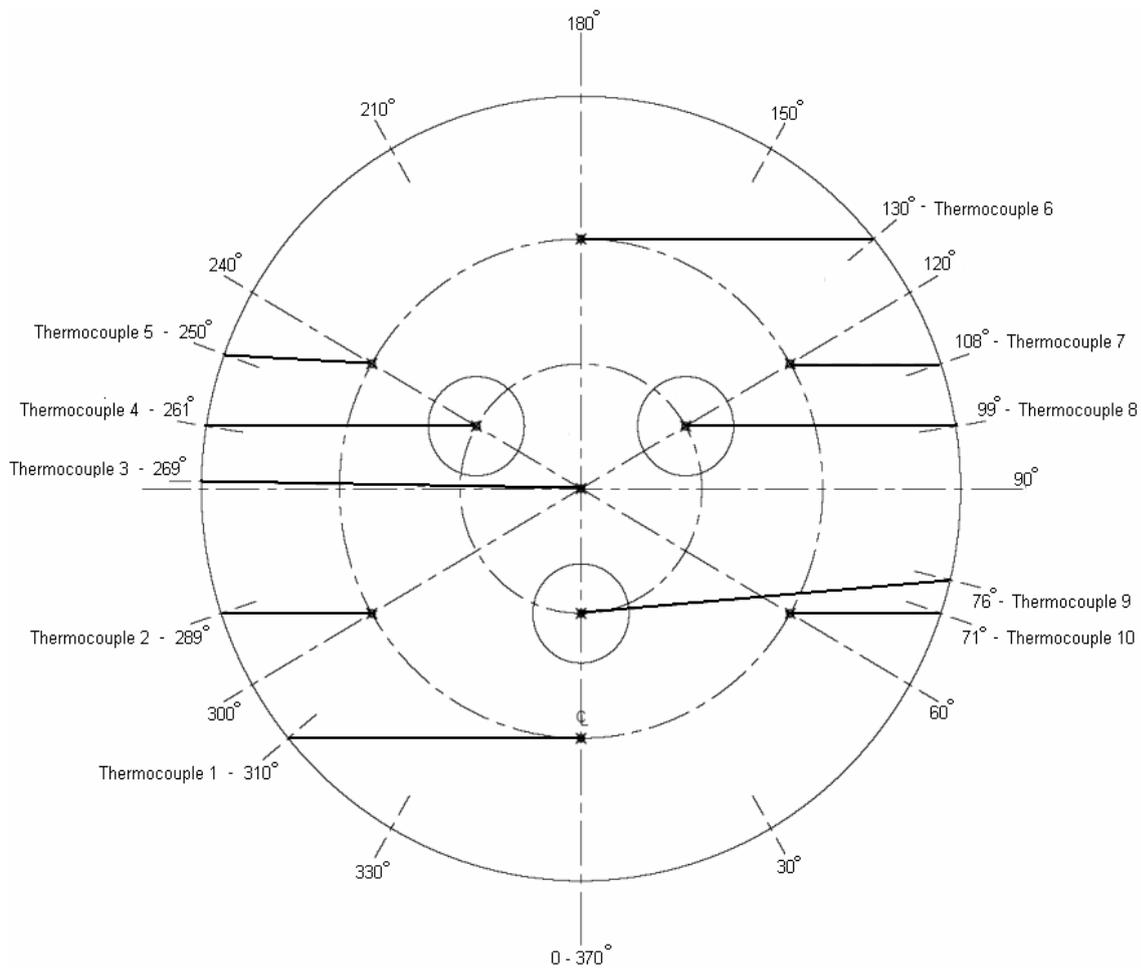
Figure 2: Hearth thermocouple layout
