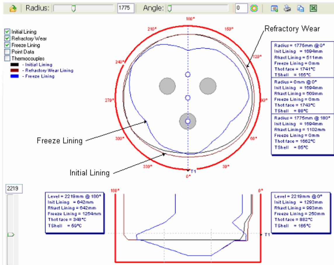
Figure 7: Lining Display Screen
