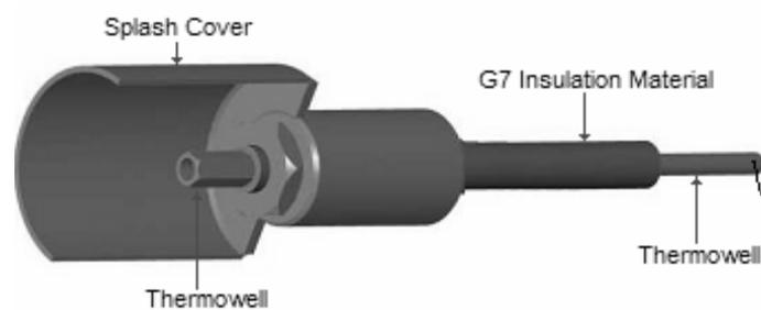
Figure 3: Insulating bush and thermo well arrangement
