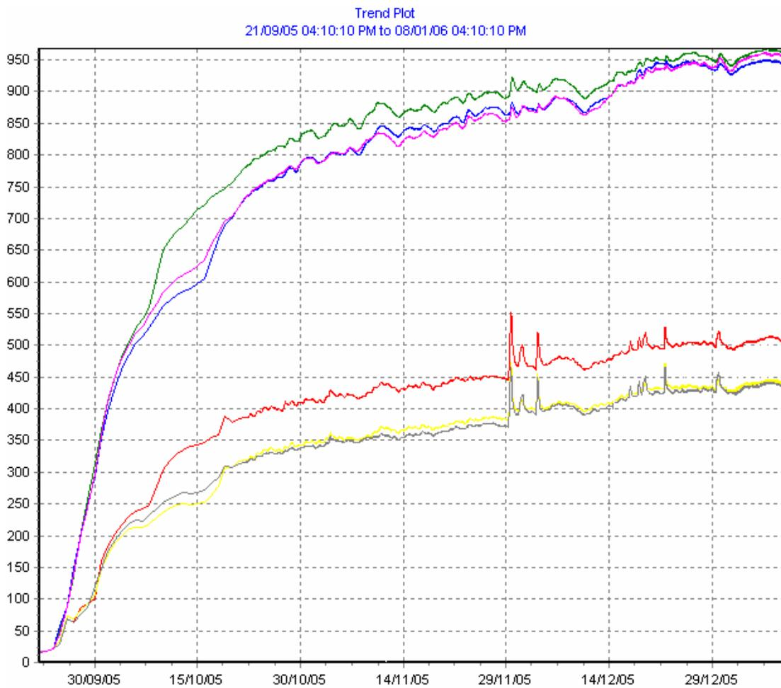
Figure 9: Furnace hearth thermocouple trends
