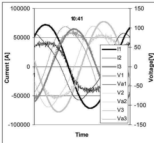
Figure 8: Snapshots of current and voltage waveforms at the start of the manual operating period. The time span is just over one AC period = 20 ms
