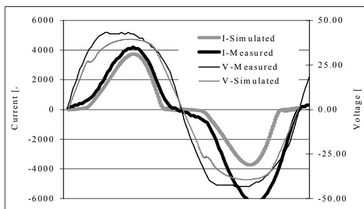
Figure 6: Current and voltage waveforms measured on the pilot furnace after the charge was melted, compared to MFD simulations for a 2 cm long arc. The time span is one AC period = 20 ms for a 50 Hz AC power source
