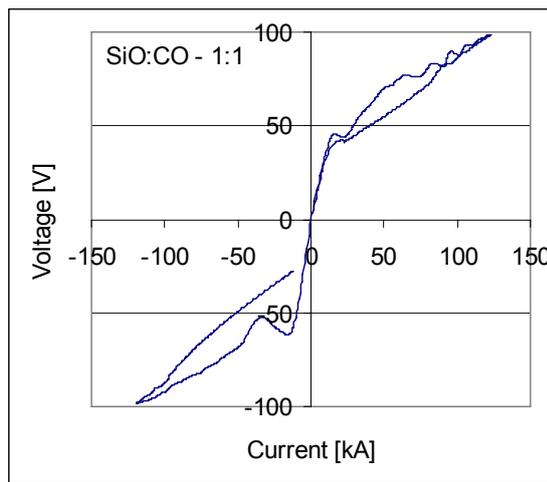
Figure 19: Lissajous figure for a simulated 5 cm long arc in SiO-CO atmosphere
