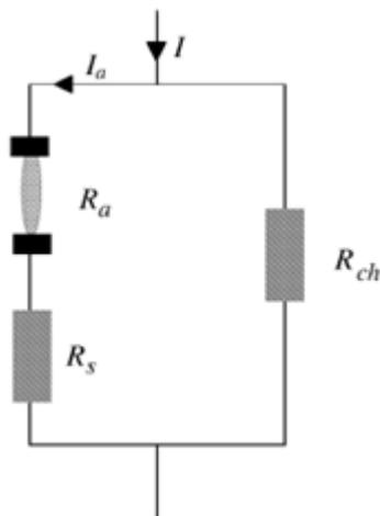
Figure 3: Schematic drawing of a configuration with a conducting charge resistance in parallel to the arc
