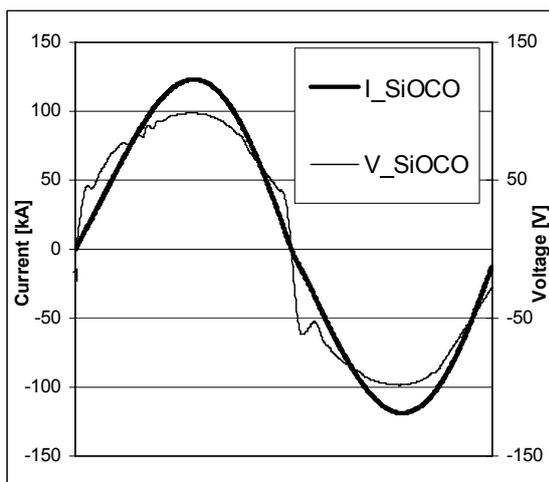
Figure 18: Current and voltage waveforms obtained from MFD simulations with SiO-CO
