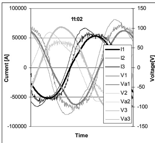
Figure 10: Electrode 1 has been raised again, the current has decreased further and the voltage increased correspondingly. The time span is one AC period = 20 ms
