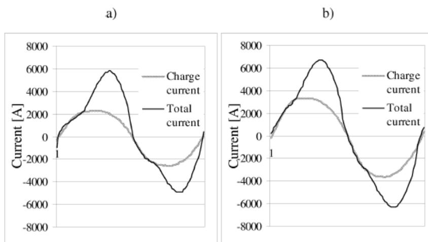
Figure 5: Current waveforms as a function of time for 20 ms at two different instances of time compared to charge current assumed to be proportional to the voltage waveforms. The upper limit of the charge current shown in these figures (53% for a) and 60% for b)), are obtained by assuming that there is no arc conduction close to zero current
