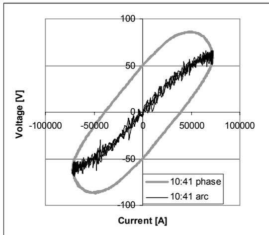
Figure 12: Lissajous figure from the first snapshot of electrode 1. The oval figure is the measured current as a function of measured voltage, while the black curve in the centre is the corrected arc voltage  $V_a$  as a function of current
