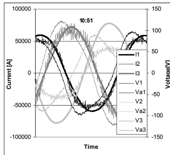
Figure 9: Electrode 1 has been raised, the current in phase 1 (black thick line) has decreased and voltage increased
