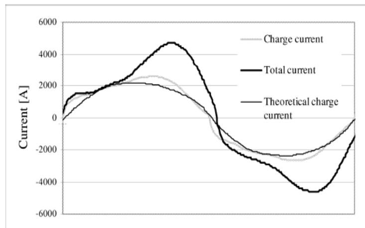
Figure 4: Current waveform during the early part of Si-metal production in the pilot furnace. The time span is one AC period = 20 ms. For comparison, the maximum linear charge current in parallel to the arc is drawn into the figure. This current is proportional to the phase voltage. In addition a similar parallel current proportional to the coke bed current as shown in Figure 1 is drawn into the figure
