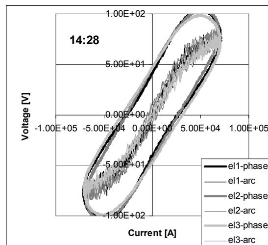
Figure 17: Lissajous curves for all three phases measured at random
