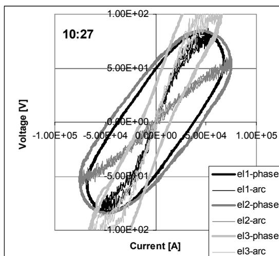
Figure 16: Lissajous curves for all three phases measured at random
