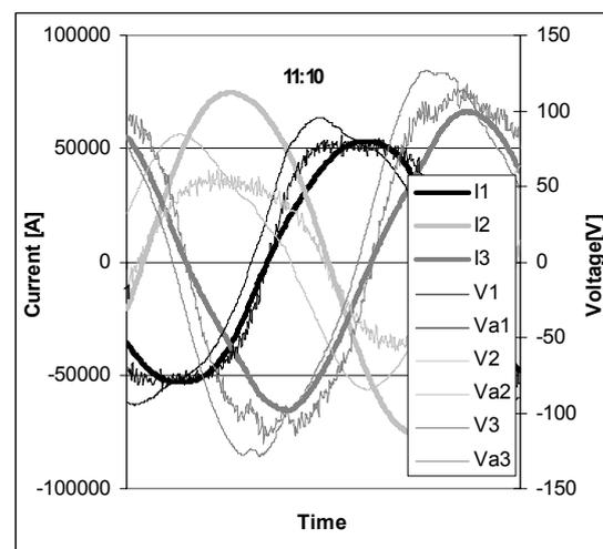
Figure 11: The same as Figure 10, after further raising of the electrode. The time span is one AC period = 20 ms
