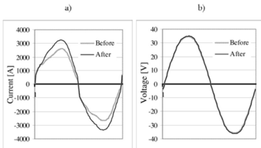
Figure 1: Current a) and voltage b) waveforms as a function of time during the heating-up of the furnace, when the electrode is in direct contact with a coke bed. The figures compare the waveforms before and after the addition of coke to the bed. As the power source is 50Hz AC, the span of the timescale is up to 20 ms
