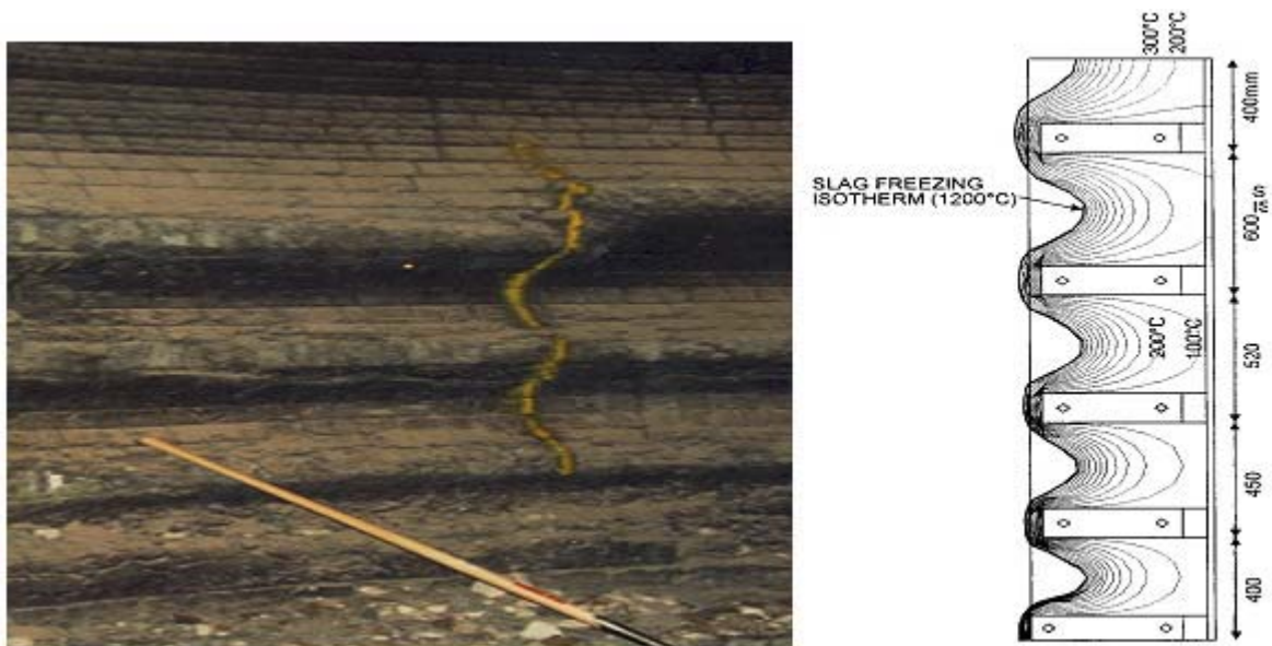
Figure 3. Comparison showing the thermal equilibrium erosion profile in a furnace (left) and that predicted by the computational model (right).
