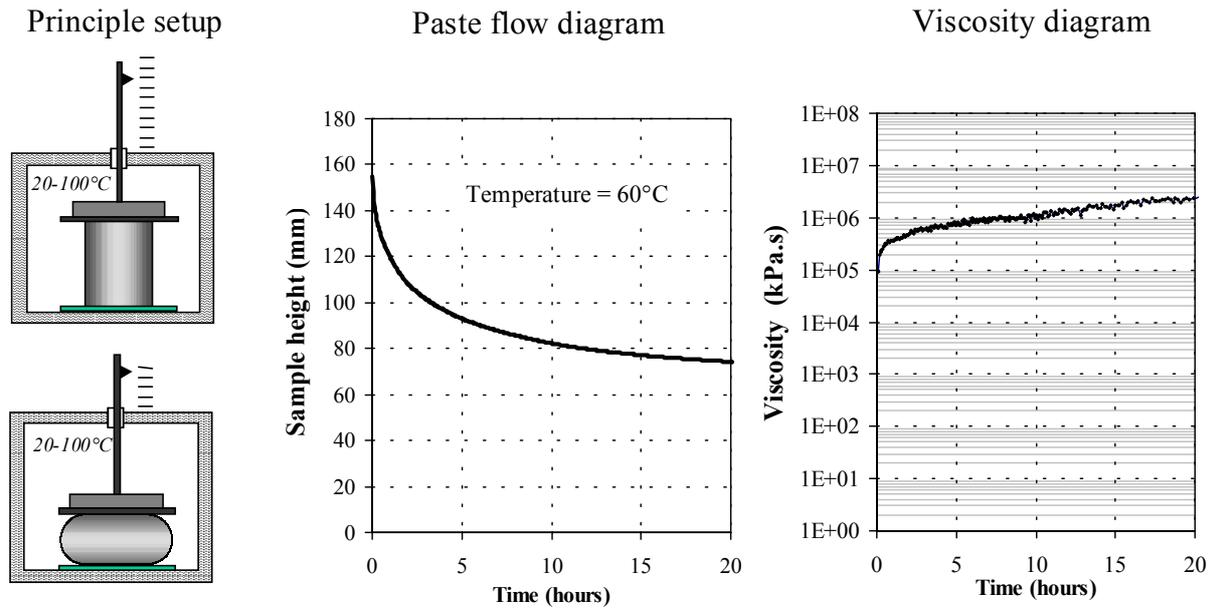
Figure 1. Flow test and viscosity measurement of a paste cylinder or “a single briquette”. The weight placed on top of the cylindrical sample ( $\varnothing$  0.17 m and  $h_0 = 0.16$  m) equals the pressure from a column of approximately 2.5 m paste cylinders.
