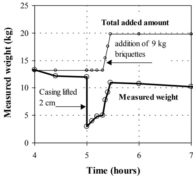
Figure 11. Results from friction test at 70°C in small electrode diameter,  $\varnothing$  0.17 m.
