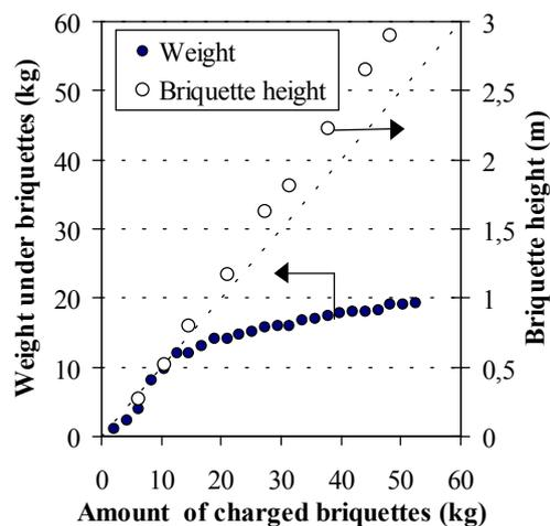
Figure 10. Result from friction test (at 20°C) in small electrode diameter,  $\varnothing$  0.17 m.
