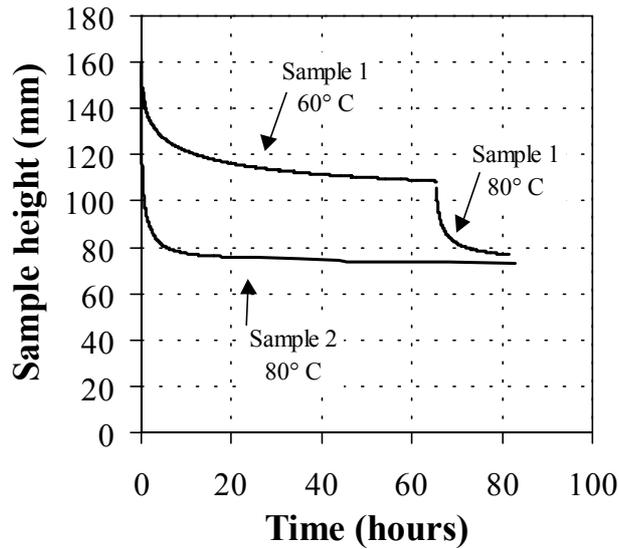
Figure 5. Comparison of flow curve at 80°C with a curve obtained in “two step test”; 65 h at 60°C followed by 15 h at 80°C.
