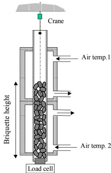
Figure 9. Setup for measurement of friction effects between paste Briquettes and steel casing. The electrode diameter is  $\varnothing$  0.17 m.
