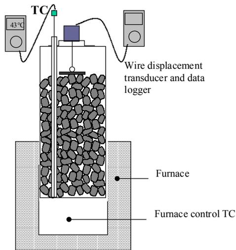
Figure 14. Setup of flow measurement of briquette bed in laboratory furnace with temperature gradient. Diameter  $\varnothing$  0.5 m.
