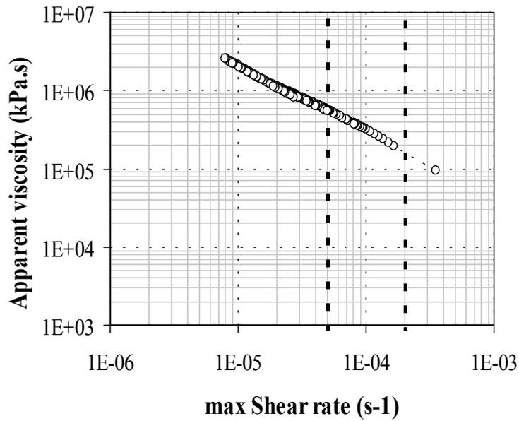
Figure 3. The apparent viscosity and shear rate relationship in electrode paste.
