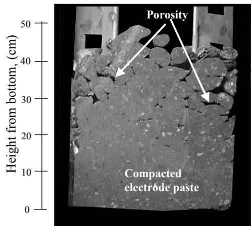
Figure 16.  $\varnothing$  0.5 m diameter electrode with briquette cut after testing according to Figure 14 and 15.
