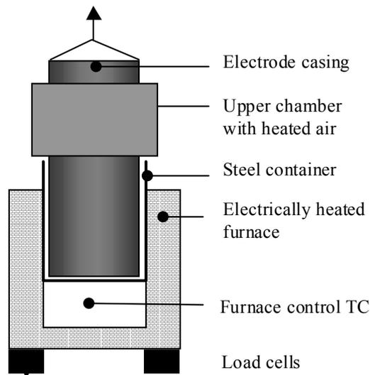
Figure 12. Test setup for briquette flow and friction testing inside 0.5 m diameter electrode.
