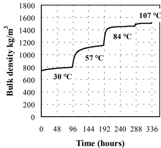
Figure 7. Compaction diagram of briquette bed at different temperature levels. High weight, 123 kg (6 kPa) on top of briquette bed. The paste’s plasticity was 22 %.
