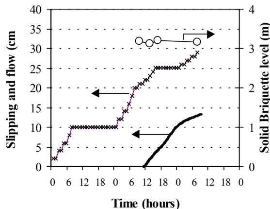
Figure 18. Measured briquette bed movement in a  $\varnothing$  1.4 m diameter industrial electrode (FeMn). The temperature on top of briquettes was 40°C.
