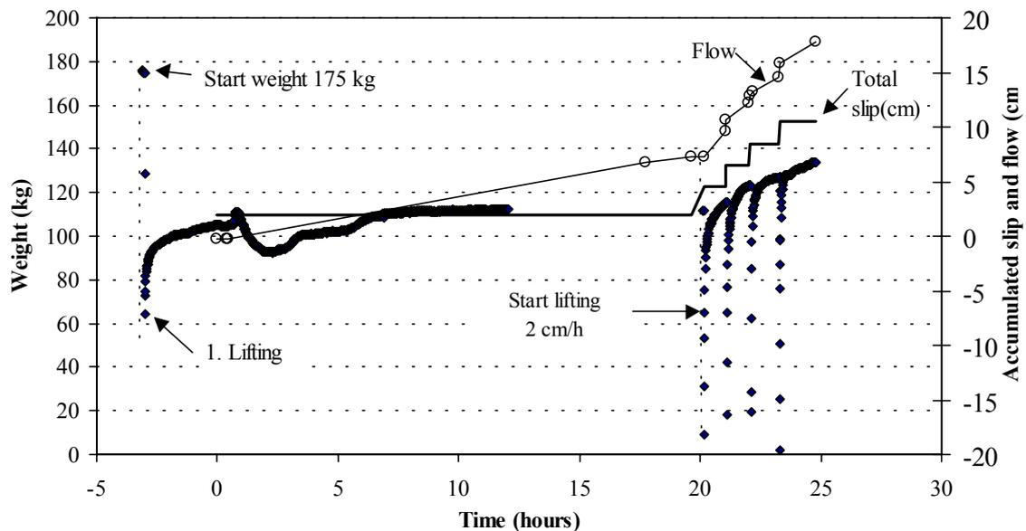
Figure 13. Friction and briquette flow test in  $\varnothing$  0.5 m diameter electrode. The flow is measured as the relative downward movement of the top of the briquette bed. Furnace temperature set point  $90^{\circ}\text{C}$  at time = 0.
