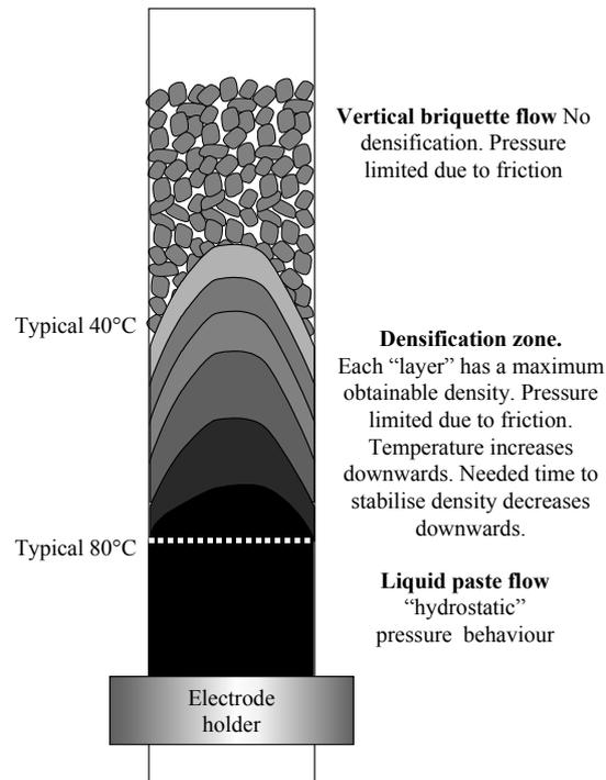
Figure 19. Schematic model of the flow and melting mechanism in upper part of a normal briquette column. Temperature for complete densification is suggested to be  $\approx 80^{\circ}\text{C}$  but depends on parameters as pitch softening point and amount.
