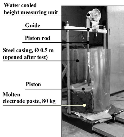
Figure 6. Pilot scale setup for flow test of briquettes in Ø 0.5 m diameter electrode. Weight is placed on top of the steel piston. The chamber temperature is changed in steps letting the paste briquette compaction stabilize at each temperature.
