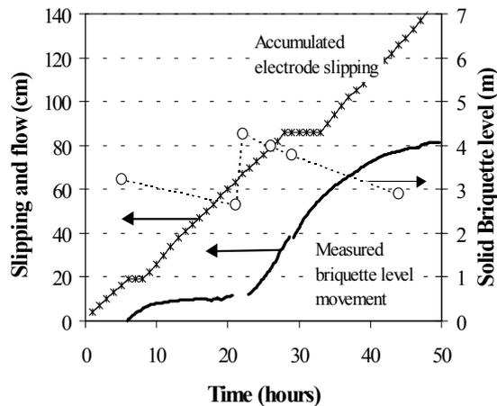
Figure 17. Measured briquette bed movement in  $\varnothing$  1.15 m diameter industrial electrode (75% FeSi). Temperature on top of briquettes was 70-80°C. Briquette was charged at time = 20 hours.
