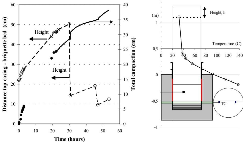
Figure 15. Flow and density test in furnace with temperature gradients. The paste flow (height = distance top casing to briquette bed) was followed by logging data from a wire displacement transducer. Briquettes were recharged twice. Furnace set point was 200°C.
