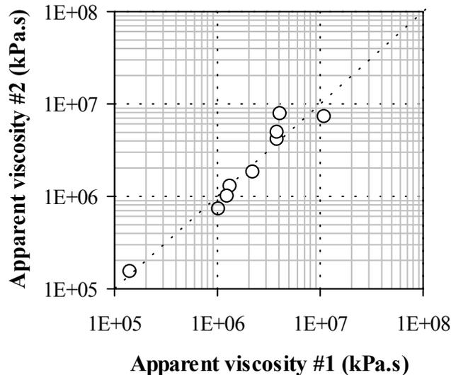
Figure 2. Isoplot of measured apparent viscosity (0.5 h). Different pastes are measured with two parallel samples. Ideal measuring system gives points on the diagonal line. Method in Fig.1.
