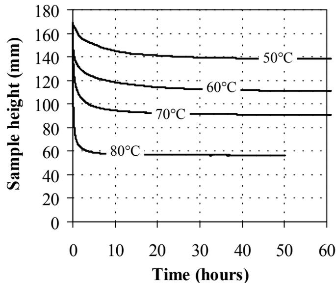
Figure 4. Temperature effect on paste flow. The paste used in this test has a lower plasticity than the paste tested in Figure 1.
