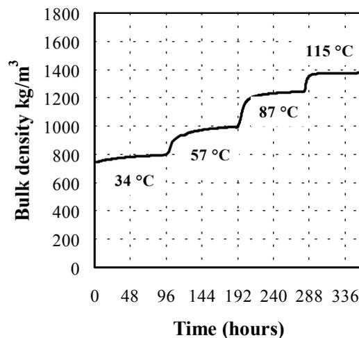
Figure 8. Compaction diagram of briquette bed at different temperature levels. Low weight, 16 kg, (0.8 kPa) on top of briquette bed. The paste's plasticity was 22%.
