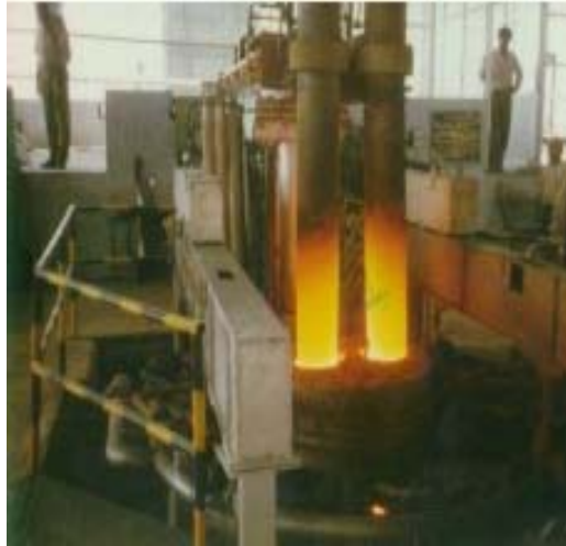
Figure 5. The two electrode DC Ladle Refining Furnace in action.
