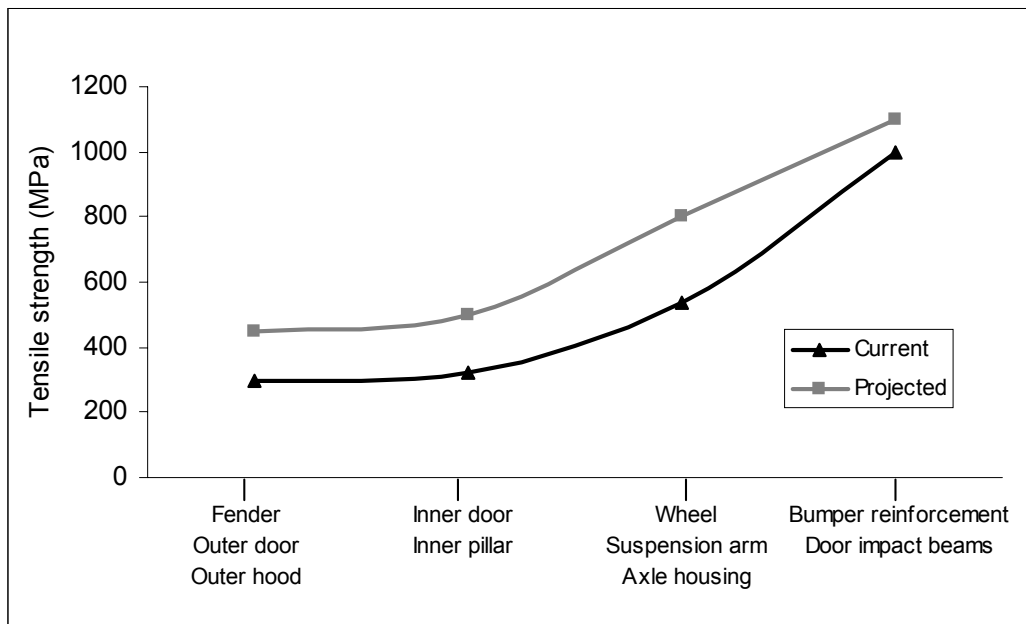
Figure 2. Tensile strength of high strength steel sheets selected for automobile body parts manufacture[8]. Current (at the time, prior to 1994) and projected values are shown.
