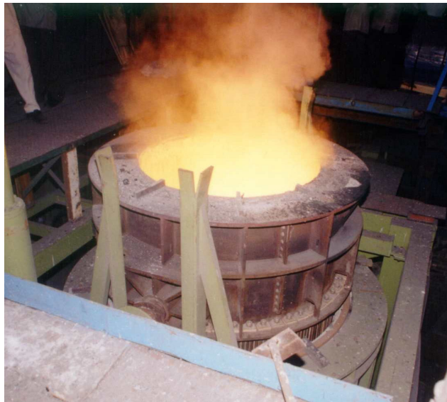
Figure 8. View of 15 t, 1500kW Induref operating at R.L. Steels Ltd. Aurangabad, India.
