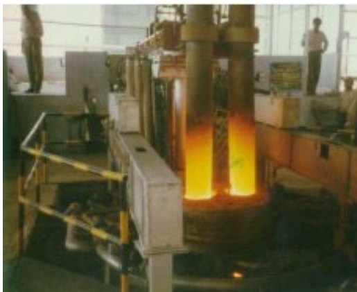
Figure 3. View of Double Electrode DC Ladle Refining Furnace.
