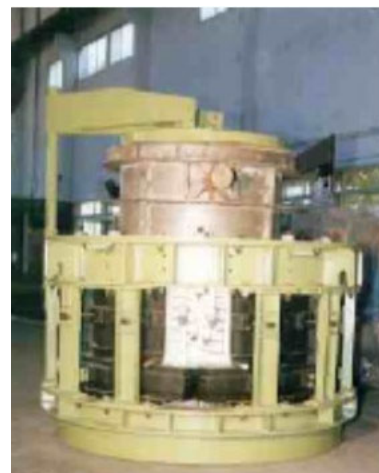
Figure 4. View of 1.5t Induction Ladle Refining Furnace used for trials.
