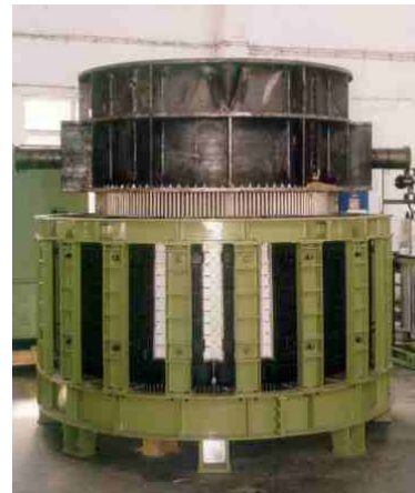
Figure 6. 15 t Capacity Induction Ladle placed in an Induction Coil Assembly.
