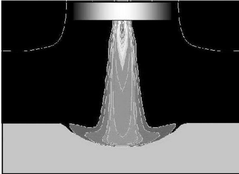
Figure 4. Assumed spherical depression created by a moving arc.
