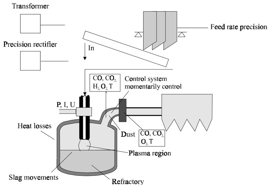
Figure 5. Set-up of the MEFOS 3 MW DC arc furnace.
