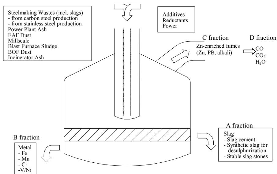
Figure 7. Recovery of materials from a complex waste using DC furnace.
