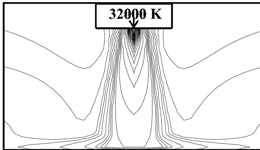
Figure 2. Temperature contours in the arc. The arc current is 36kA and the arc length 25 cm. Each line represents 1500 K.
