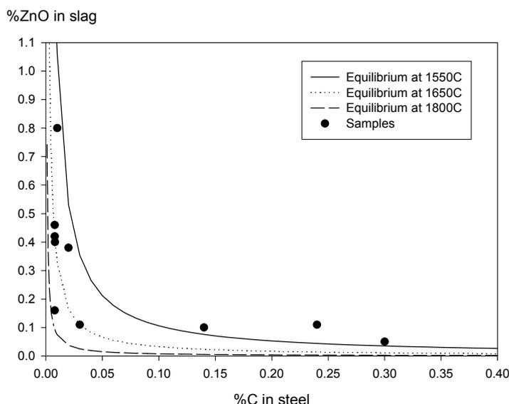
Figure 8. Equilibrium between ZnO-content in slag and C-content in steel.
