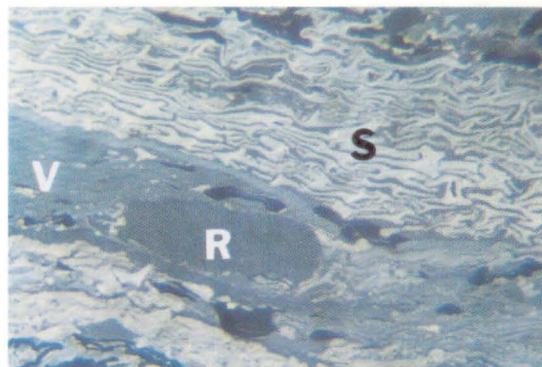
Picture 6 Photomicrograph of Slask coal showing (V) Vitrinite, (R) Resinite and (S) Semifusinite. Magn. X 450 in light microscope.
