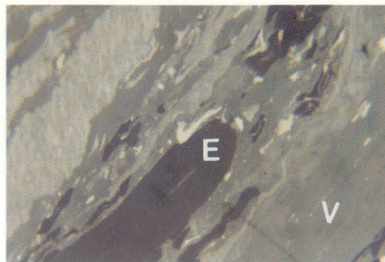
Picture 2 Polished Pokoj coal sample in oil showing (V) Vitrinite, and (E) Exinite. Magn. X 450 in light microscope.
